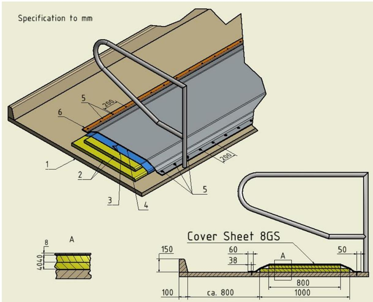
*Legend: 1 Concrete, 2 Composite foam, 3 Plastic foil, 4 Cover sheet 8GS, 5 Mounting, 6 Angle bar*
