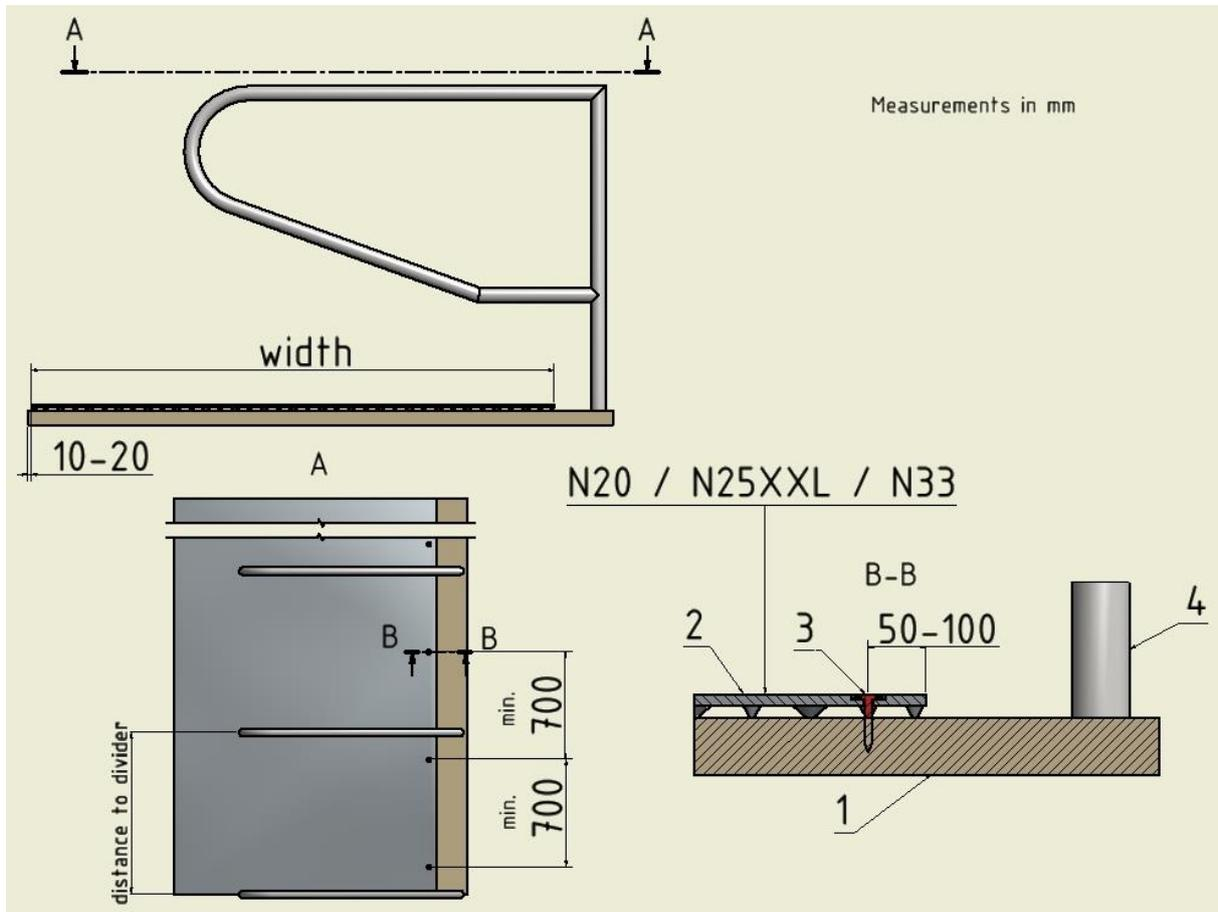
Legend: 1 Concrete, 2 Lining N20/N25/N33, 3 Mounting, 4 Separating Frame
